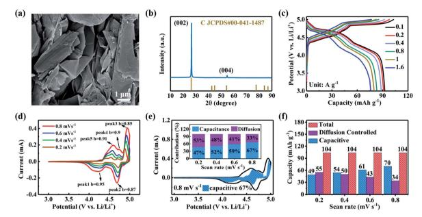
Fig. 3 (a) SEM image and (b) XRD patterns of the as-prepared EG; (c) charge/discharge profiles at varied currents rates and (d) CV curves at varied scan rates of the EG electrode; (e) CV curves with capacitive contribution (shadowed area) at 0.8 mV s<sup>-1</sup> (insert: the contribution ratio of diffusion-controlled and capacitive *versus* scan rate) and (f) capacitive, diffusion-control and total capacities for varied scan rates of the EG electrode.
