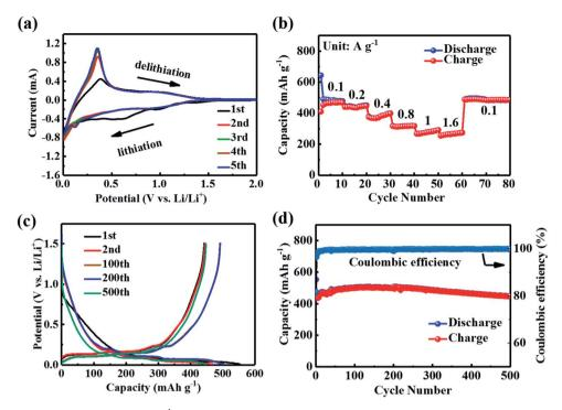
Fig. 2 (a) CV curves at a scan rate of 0.1 mV s<sup>-1</sup>, (b) rate performance at varied currents, (c) charge/discharge profiles and (d) long cycling performance at 100 mA g<sup>-1</sup> of the Si/C electrode.
