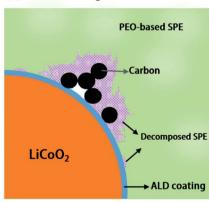
(b) Particles coating cathode/SPE interface
