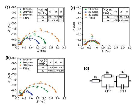
Fig. 4 EIS spectra of ASSLBs with (a) bare  $LiCoO_2$  electrode, (b) LCO-coating protected  $LiCoO_2$  electrode, and (c) LCO + CB-coating protected  $LiCoO_2$  electrode after 10, 20, and 30 cycles of charge/discharge. The inset tables show the critical frequency values on top of the high frequency semi-circle ( $F_a$ ) and low frequency semi-circle ( $F_c$ ) at different cycles of charge/discharge, respectively. (d) The equivalent circuit for fitting the EIS spectra.
