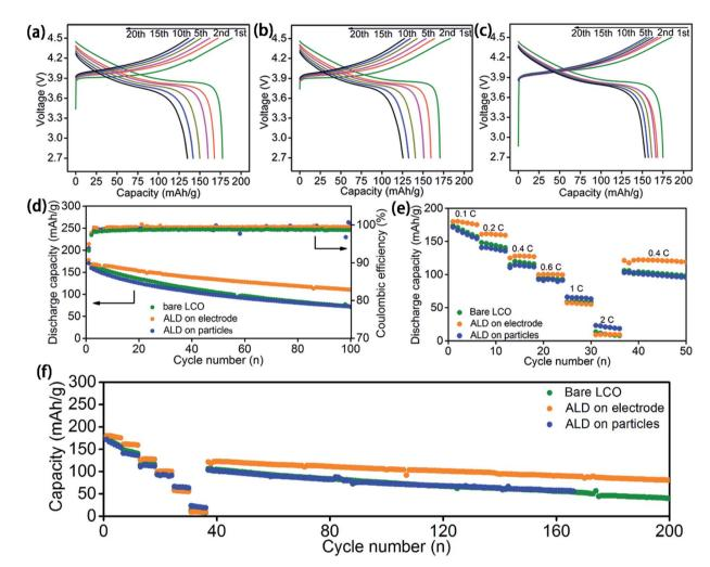
Fig. 3 Charge/discharge profiles of ASSLBs with (a) bare  $LiCoO_2$  electrode, (b) LCO-coating protected electrode, and (c) LCO + CB-coating protected electrode at 0.2C and 60 °C. Corresponding (d) cycling performance, (e) rate performance, and (f) long-term cycling performance after rate performance testing for ASSLBs with different  $LiCoO_2$  electrodes at 60 °C.
