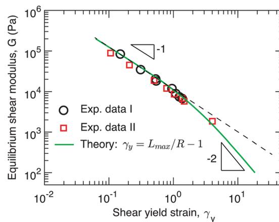
**Fig. 3** Dependence of stiffness on yield strain. The symbols are experimental data points extracted from Fig. 2a (circles) and Fig. 2b (squares). Solid line: theoretical prediction for the dependence of network stiffness  $G$  on the shear yield strain  $\gamma_y$  calculated based on  $\gamma_y = L_{\text{max}}/R - 1$  (eqn (1)), where both  $L_{\text{max}}$  and  $R$  are determined by the  $G$  (eqn (2), (3), (9), and (11)).
