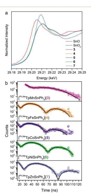
Fig. 5 (a) The XANES spectra at the Sn K-edge for polycrystalline samples of 3–7 (29 200.4 eV for Sn metal reference), including SnO and SnO $_2$  standards, measured at 25 K. (b)  $^{119}$ Sn synchrotron Mössbauer spectra of 3–7 collected at 60 K. Open circles represent the experimental data, and the black lines represent fits to the spectra.
