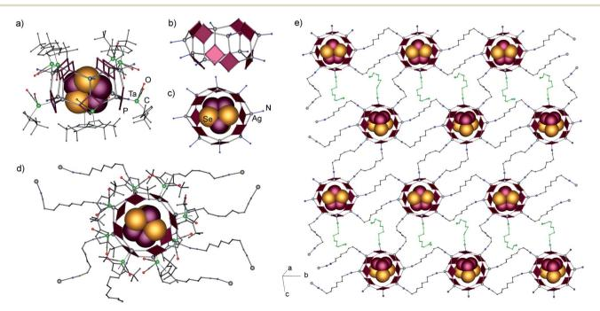
Fig. 4 (a) Supramolecular node, (b) its 40-vertex inorganic core (c) containing a  $P_4Se_3$  guest molecule, (d) node with outgoing linkers, (e) 2D network of interconnected nodes in 7. The guest is depicted in the space-filling model. Non-coordinating linker units are highlighted in green. {Cp"Ta(CO)<sub>2</sub>} fragments and counter-anions are omitted for clarity.
