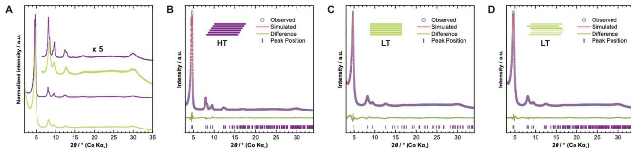
Fig. 4 (A) Comparison of X-ray diffraction patterns of HT (purple) and LT (green) collected with Co  $K\alpha_1$  radiation. (B) Diffraction pattern of HT with best-obtained fit by Rietveld refinement assuming unidirectional slip stacking. (C) Diffraction pattern of LT with best-obtained fit by Rietveld refinement assuming eclipsed stacking and (D) random stacking.
