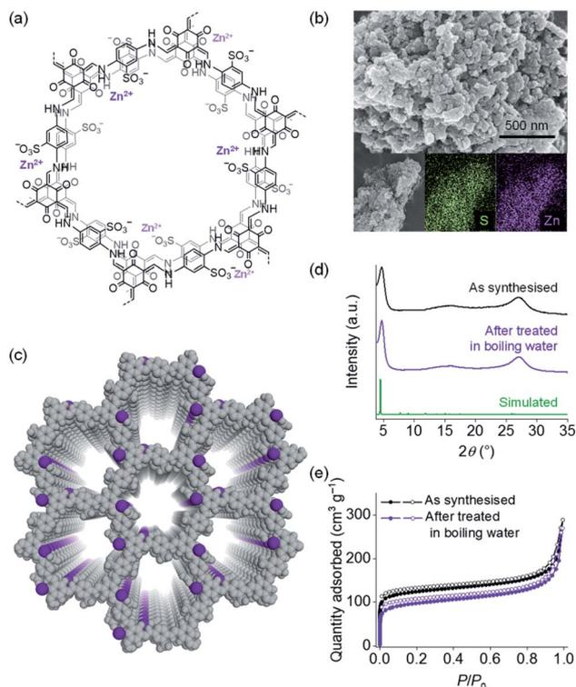
Fig. 1 (a) Chemical structure, (b) SEM and EDS mapping (for S and Zn) images, (c) structural model (Zn<sup>2+</sup>: purple, TpPa-SO<sub>3</sub><sup>-</sup>: grey), (d) XRD patterns and (e) N<sub>2</sub> gas isotherms of TpPa-SO<sub>3</sub>Zn<sub>0.5</sub>.
