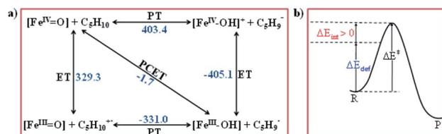
Fig. 4 (a) Relative thermodynamic free energies between the  $\text{Fe}^{\text{IV}}=\text{O}$  unit and its hydroxo complexes (all energies are in  $\text{kJ mol}^{-1}$ ) and (b) the relationship between the barrier ( $\Delta E^\ddagger$ ), the deformation energy of reactant ( $\Delta E_{\text{def}}$ ) and the interaction energy  $\Delta E_{\text{int}}$  at the transition state:  $\Delta E_{\text{int}} > 0$ .
