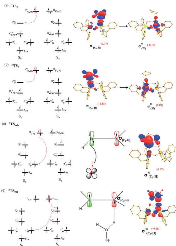
Fig. 3 Electron shift diagrams of  $\text{I}^{\text{-}}\text{TS}_{\text{H}}$  for both (a)  $\text{I}^{\text{-}}\text{TS}_{\text{Hhs-hs}}$ , (b)  $\text{I}^{\text{-}}\text{TS}_{\text{Hhs-hs}}$ , (c)  $\text{Ia}^{\text{-}}\text{TS}_{\text{rebhs-hs}}$  and (d)  $\text{Ib}^{\text{-}}\text{TS}_{\text{2Hhs-hs}}$  with SNOs and their occupation (noted in parentheses).
