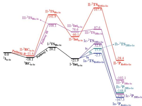
Fig. 6 Potential energy surface computed (energies are in  $\text{kJ mol}^{-1}$ ) for C–H activation of cyclopentane by species  $^2\text{I}_{\text{hh-hs}}$  comparing the lowest estimate of barrier heights obtained from various pathways computed in Scheme 2.
