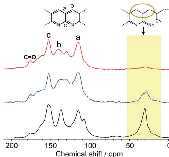
Fig. 5 Solid-state <sup>13</sup>C NMR spectra of LP prepared from neat PAN (black) and liberated from **1a** (red) and **1b** (blue).
