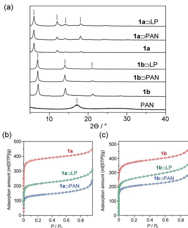
Fig. 3 (a) PXRD patterns of PAN, **1**, **1**⊃PAN, and **1**⊃LP. (b and c) N<sub>2</sub> adsorption isotherms of (b) **1a**, **1a**⊃PAN, **1a**⊃LP, (c) **1b**, **1b**⊃PAN, and **1b**⊃LP.
