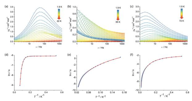
Fig. 2 Frequency dependence of the imaginary component of the AC susceptibility,  $\chi''$  versus  $\nu$ , in zero DC field for (a) 1, (b) 2 and (c) [3][B(C<sub>6</sub>F<sub>5</sub>)<sub>4</sub>] at the temperatures indicated, and the temperature dependence of the relaxation time as  $\ln \tau$  versus  $T^{-1}$  for 1 (d), 2 (e) and (f) [3][B(C<sub>6</sub>F<sub>5</sub>)<sub>4</sub>].
