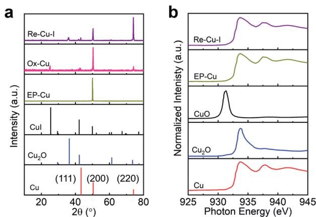
Fig. 2 Structural characterization of EP-Cu, Ox-Cu and Re-Cu-I. (a) GIXRD patterns of Re-Cu-I (purple), Ox-Cu (pink), EP-Cu (yellow) and reference samples CuI (black, PDF#06-0246),  $\text{Cu}_2\text{O}$  (blue, PDF#05-0667), and Cu (red, PDF#04-0836). (b) Cu L-edge XAS spectra of Re-Cu-I (purple), EP-Cu (yellow) and reference samples CuO (black),  $\text{Cu}_2\text{O}$  (blue) and Cu (red).
