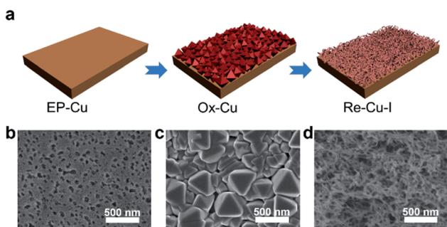
Fig. 1 Schematic illustration and morphology characterization of the surface reconstruction process. (a) Scheme of the electrochemical redox reconstruction process. SEM images of EP-Cu (b), Ox-Cu (c) and Re-Cu-I (d).
