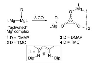
Scheme 1 Previously reported syntheses of magnesium deltate complexes, 3 and 4 (Dip = 2,6-diisopropylphenyl, DMAP = 4-dimethylaminopyridine, TMC =  $C\{(MeNCMe)_2\}$ ).
