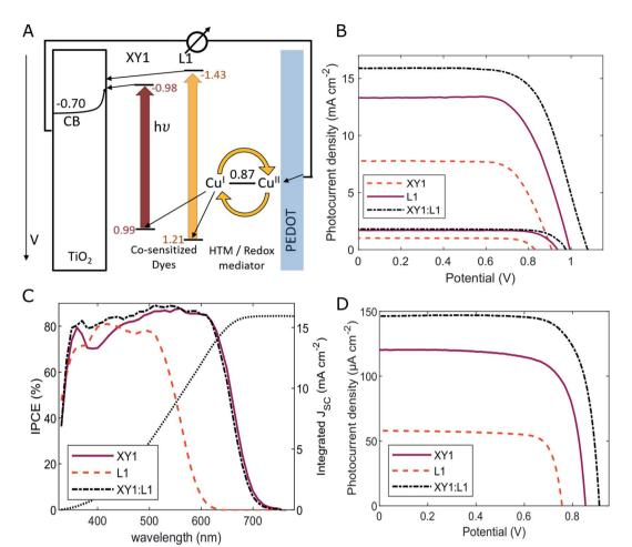
Fig. 2 (A) Working principle of the XY1:L1-sensitized DSC. (B) Photovoltaic performance under simulated sunlight (AM 1.5G, 100 mW cm $^{-2}$ ) and 10% sunlight, (C) incident photon to current conversion efficiency spectra (IPCE), and (D) photovoltaic performance under 1000 lux fluorescent light (303.1  $\mu$ W cm $^{-2}$ ) of XY1, L1 and XY1:L1 co-sensitized DSCs. Corresponding parameters are listed in Table 1.
