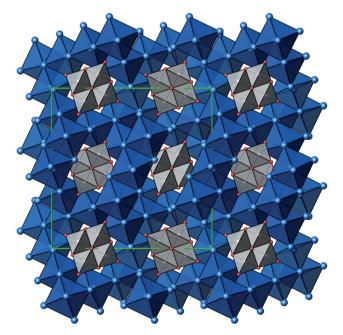
Fig. 3 Projection of the crystal structure of  $Ag_{16}B_4O_{10}$ , view along [001], with margins of the unit cell (green). Color code: Ag (blue spheres), B (grey spheres), O (red spheres), blue octahedra ( $Ag_6$ ), grey tetrahedra ( $BO_4$ ).
