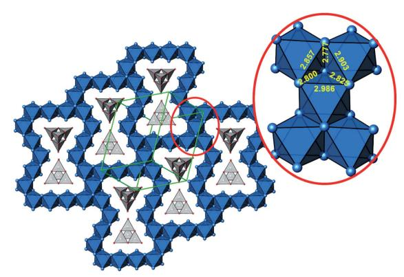
Fig. 4 Cut-out of the crystal structure of Ag<sub>16</sub>B<sub>4</sub>O<sub>10</sub>, view along [121]. Magnification (red circle) highlights a block consisting of five edge sharing octahedra with Ag-Ag distances labeled. Same color code as in Fig. 3.
