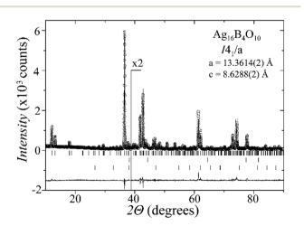
Fig. 1 PXRD pattern of the  $Ag_{16}B_4O_{10}$  sample, showing the observed (circles), Rietveld fit (black line) and difference curve (gray line). The upper, middle and bottom bars mark the reflections for  $Ag_{16}B_4O_{10}$ , Ag and  $Ag_2O$ , respectively. The intensity is doubled in the inset for clarity.
