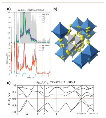
Fig. 7 (a) Total and atom-projected density of states, (b) isosurface  $(0.04 \text{ e}^{-} \text{ Å}^{-3})$  of the electron density generated by the disperse bands below the Fermi level ( $E_F - 1.44 \text{ eV}$  to  $E_F$ ), (c) bands at  $E_F$ .
