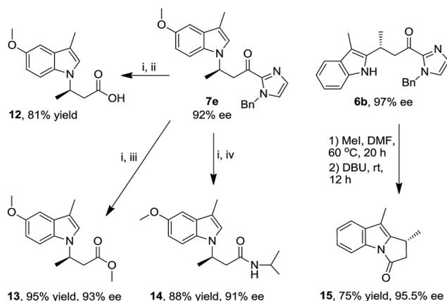
Scheme 2 Synthetic elaboration studies. Reaction conditions: (i) MeI, DMF, 60 °C, 20 h; (ii) DBU,  $\text{H}_2\text{O}$ , rt, 4 h; (iii) DBU,  $\text{CH}_3\text{OH}$ ,  $\text{CH}_2\text{Cl}_2$ , rt, 6 h; (iv) DBU,  $i\text{PrNH}_2$ , rt, 12 h.
