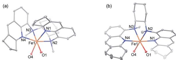
Fig. 1 ORTEP drawings of (a) **1e** and (b) **1f** (30% probability ellipsoids) with the omission of H atoms and OTf<sup>-</sup> ligands except O atoms bound to Fe<sup>II</sup>.
