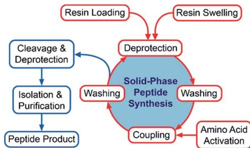
Fig. 1 Overview of the SPPS cycle and subsequent deprotection, work-up and purification steps. The present review focuses on technical aspects of the SPPS cycle (shown in red) while cleavage, deprotection, isolation and purification steps (shown in blue), are only briefly touched upon.
