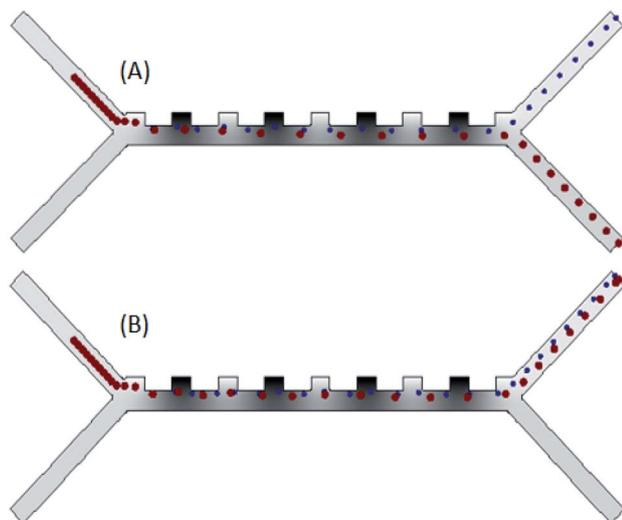
Fig. 7 (A) Analysis results of the separation of blood cells in the channels of the microfluidic chip (B) blood cells in the channels of the microfluidic chip come out of a single channel.
