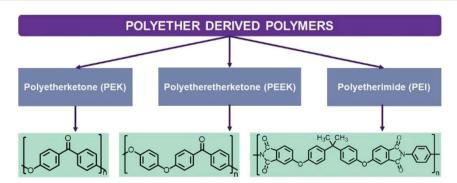
Fig. 10 Chemical structure for PEI, PEK and PEEK which are polyether-based polymers; chemical structures were drawn by the author.
