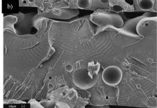
Fig. 12 SLS of PC under (a) 0.036 J mm<sup>-1</sup> and (b) 0.094 J mm<sup>-1</sup> laser density, respectively.<sup>170</sup> Reprinted with permission from Elsevier: *Journal of Materials Processing Technology*, Copyright 1999, License number: 4838261399886.
