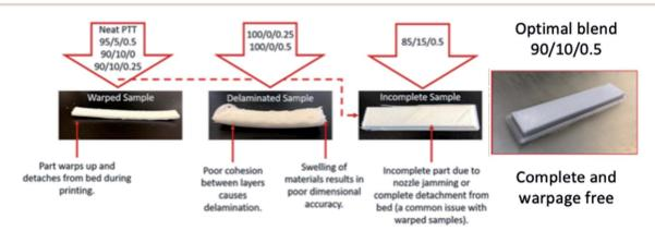
Optimization of PTT/impact modifier/chain extender blends to make complete samples as novel use for PTT in 3D printing.6
