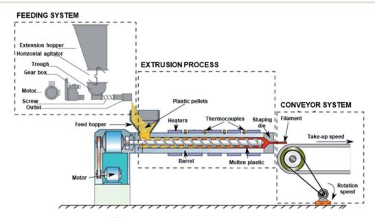
Fig. 1 Extrusion set-up for filament processing.<sup>35</sup> Reprinted with permission from Elsevier: Additive Manufacturing, Copyright 2020, License: 4838260364616.
