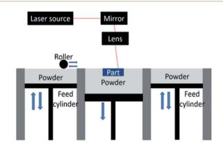
Fig. 4 Selective laser sinter schematic.<sup>46</sup> Reprinted with permission from Elsevier: *Journal of Manufacturing Processes*, Copyright 2020, License: 4743141319375.
