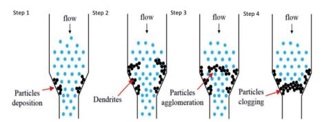
Fig. 13 Modelled clog formation for PC composites *via* FFF.<sup>171</sup> Reprinted with permission from John Wiley and Sons: *Journal of Applied Polymer Science*, Copyright 2019, License: 4732631260702.
