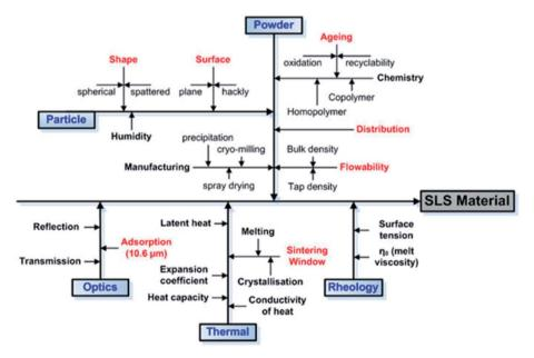
Fig. 5 Parameters of powder and processing conditions that influence SLS printed products.<sup>128</sup> Reprinted with permission from Cambridge University Press: *Journal of Materials Research*, Copyright 2014, License: 4840231185789.
