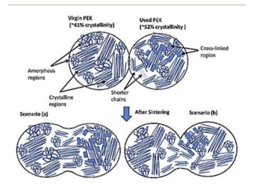
Fig. 11 Two scenarios for re-ordering between virgin and used PEK powders during SLS.<sup>48</sup> Reprinted with permission from Elsevier: *Journal of Materials Processing Technology*, Copyright 2019, License: 4632510363502.
