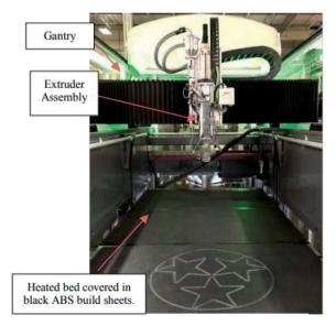
Fig. 3 Big-area-additive-manufacturing extrusion 3D printer.<sup>43</sup> Reprinted with permission from Elsevier: *Procedia Manufacturing*, Copyright 2020, License: 4743161414193.
