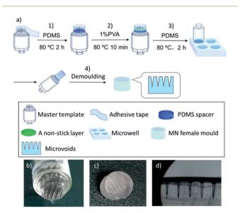
Fig. 1 (a) Microneedle female mould fabrication procedure, containing four steps: (1) preparation of the tunable master template using a PDMS spacer, (2) formation of a non-stick layer, (3) preparation of female templates, and (4) demoulding. (b) The spacer-modified master template. (c) The female mould and (d) the side view of the female mould.
