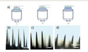
Fig. 2 (a) Length adjustment scheme. (b-d) Microneedle (MN) micrographs when using 50, 100, and 150 µL of spacer.
