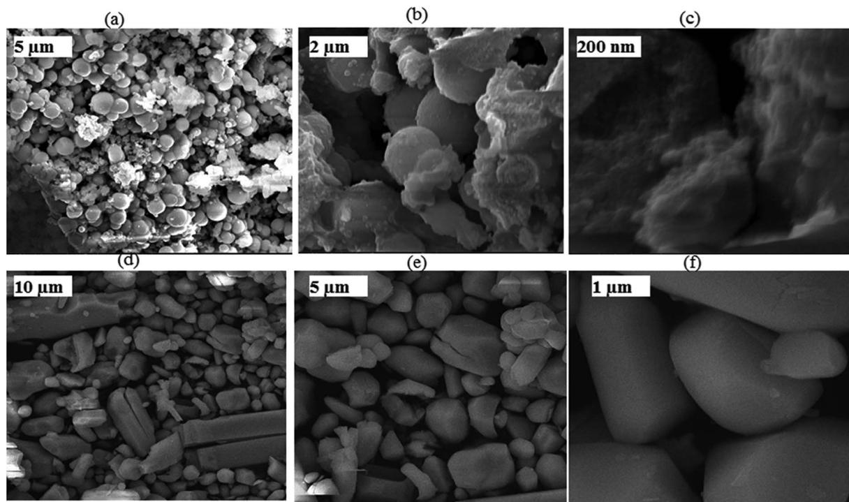
Fig. 6 (a–c) FE-SEM images of the organic template-assisted  $\text{CoMoO}_4$  at different magnifications. (d–f) FE-SEM images of the controlled sample (ethylene glycol assisted  $\text{CoMoO}_4$ ) at different magnifications.
