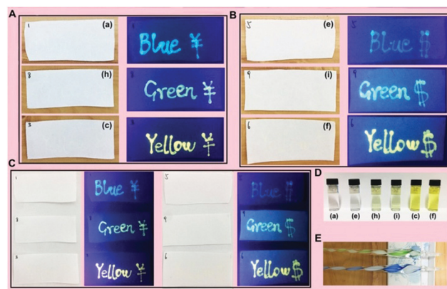
Fig. 4 Fluorescence intensity changes upon changes in temperature and solvents. (A) Application of DSA-G \subset H1-4C4P (a, h, c) and (B) DSA-G \subset H2-2C4P (e, i, f) written on filter paper, (left: under natural light, right: under ultraviolet light, \lambda_{em} = 365 nm) as tunable fluorescent inks. (C) Fluorescent inks of DSA-G \subset H1-4C4P (a, h, c) and DSA-G \subset H2-2C4P (e, i, f) on the same white paper; (a): H1-4C4P ([ H1-4C4P ] = 50 \mu M); h: DSA-G \subset H1-4C4P ([ H1-4C4P ] = 50 \mu M, [ DSA-G ] = 10 \mu M); c: DSA-G \subset H1-4C4P ([ H1-4C4P ] = 50 \mu M, [ DSA-G ] = 100 \mu M); e: H2-2C4P ([ H2-2C4P ] = 50 \mu M); i: DSA-G \subset H2-2C4P ([ H2-2C4P ] = 50 \mu M, [ DSA-G ] = 10 \mu M); f: DSA-G \subset H2-2C4P ([ H2-2C4P ] = 50 \mu M, [ DSA-G ] = 100 \mu M)). Images of (D) the solutions and (E) solution-loaded pens.
