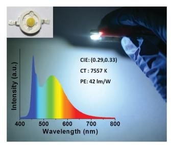
Fig. 6 Photograph of a CD-based working LED prototype utilizing a CDs@g-C<sub>3</sub>N<sub>4</sub> composite with 1 wt% CDs as a phosphor, and its emission spectra with the related characteristics. CIE: CIE color coordinates, CT: color temperature, PE: power efficiency.
