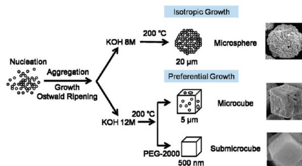
**Fig. 5** Crystal morphology control of  $\text{BiFeO}_3$  proposed by Li *et al.* and reproduced with permission.<sup>146</sup>
