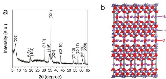
**Fig. 17** (a) XRD pattern of sodium iron oxide nanosheets synthesised under microwave irradiation at 180 °C for 5 min. (b) Crystal structure of  $Na_{2.4}Fe_{10.99}O_{16.03}$  viewed perpendicular to the  $c$  axis. The pink, red, and grey spheres correspond to Na, O, and Fe atoms, respectively. Reproduced with permission from Wu *et al.*<sup>328</sup>
