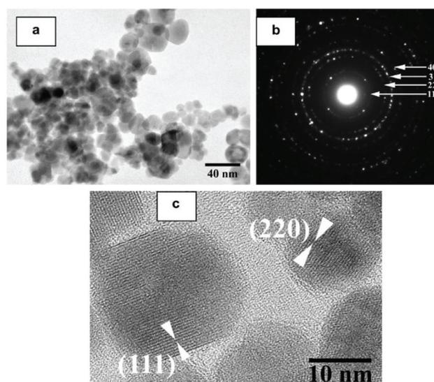
Fig. 8 (a) Bright field TEM micrograph, (b) selected area diffraction and (c) HRTEM image of hydrothermally prepared nanocrystalline Mn<sub>0.8</sub>Zn<sub>0.2</sub>Fe<sub>2</sub>O<sub>4</sub>. Reprinted with permission from Nalbandian *et al.*<sup>194</sup>
