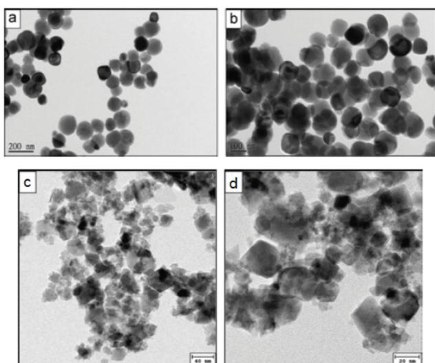
Fig. 12 CoFe<sub>2</sub>O<sub>4</sub> nanospheres (a and b) and nanocubes (c and d) synthesised in water through controlled sonochemistry at room temperature. Reproduced with permission from Abbas *et al.*<sup>256</sup>
