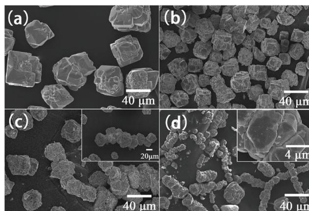
**Fig. 6** SEM images of  $\text{BiFeO}_3$  obtained by hydrothermal synthesis at 200 °C with 8 M KOH for 6 h in various magnetic fields: (a) 0 T; (b) 4 T; (c) 8 T and (d) 12 T. Reproduced with permission from Hou *et al.*<sup>151</sup>
