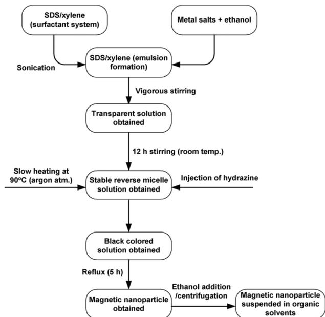
Fig. 15 Flow chart of the typical experimental procedure for the microemulsion synthesis of ferrite nanoparticles (adapted with permission from Mathew *et al.*).<sup>34</sup> SDS: sodium dodecyl sulphate.
