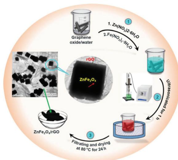
Fig. 13 Reaction scheme for formation of ZnFe<sub>2</sub>O<sub>4</sub>/graphene oxide nanocomposite using sonochemistry. Reproduced with permission from Chen *et al.*<sup>257</sup>
