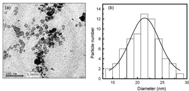
**Fig. 22** Cobalt spinel  $\text{CoFe}_2\text{O}_4$  synthesised by a modified citrate sol-gel approach: TEM morphology of the as-burnt powder (a) and corresponding grain size histogram obtained by statistical method (b). Reproduced with permission from Gass *et al.*<sup>352</sup>
