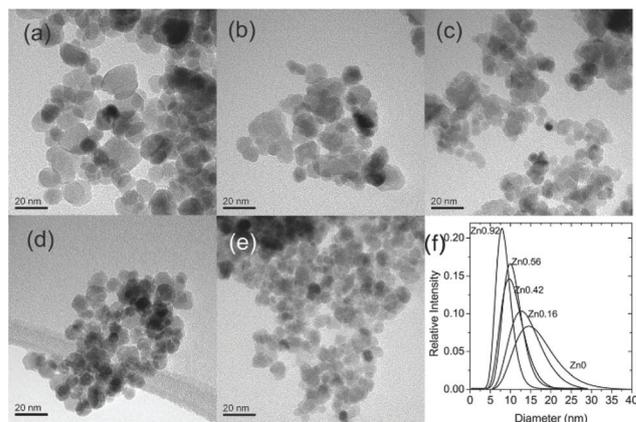
**Fig. 21** TEM images showing (a)  $\text{Zn}_0$ , (b)  $\text{Zn}_{0.16}$ , (c)  $\text{Zn}_{0.42}$ , (d)  $\text{Zn}_{0.56}$ , (e)  $\text{Zn}_{0.92}$ , and (f) size distributions of all samples prepared through bacterially-assisted synthesis. Data obtained by measurement of  $n = 200$  particle diameters per sample. Reproduced from Byrne *et al.*<sup>351</sup>
