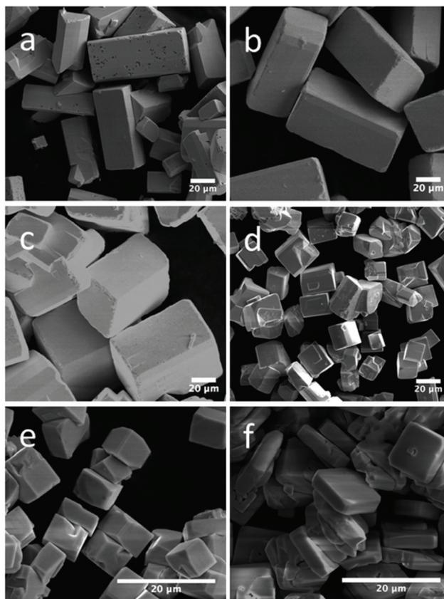
Fig. 7 SEM images of orthorhombic  $\text{YbFeO}_3$  with NaOH/KOH mixed mineraliser: (a) 25 M/0 M; (b) 20 M/5 M; (c) 15 M/10 M; (d) 10 M/15 M; (e) 5 M/20 M; and (f) 0 M/25 M. Reproduced with permission from Zhang *et al.*<sup>170</sup>
