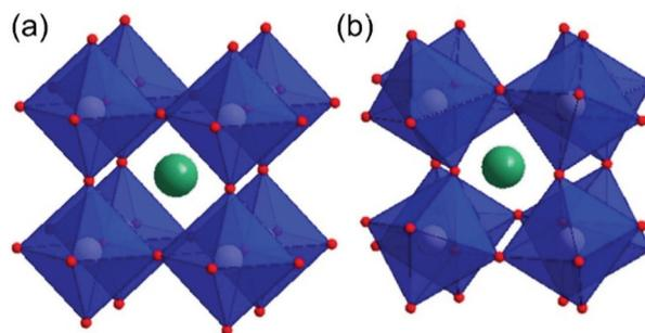
Fig. 2 The  $ABX_3$  perovskite structure (a) view of ideal cubic unit cell with blue  $[BX_6]$  octahedral and green 12-coordinate A sites and (b) the distorted orthorhombic unit cell as found for  $GdFeO_3$  where the octahedral are tilted with respect to each other.
