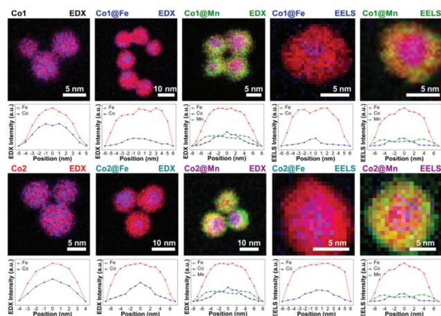
**Fig. 10** Energy-dispersive X-ray maps of metal cation concentration in core-shell nanocrystals of cobalt ferrite and manganese ferrite coated with a second spinel oxide, with line-scans below each map. Reproduced with permission from Angotzi *et al.*<sup>221</sup>
