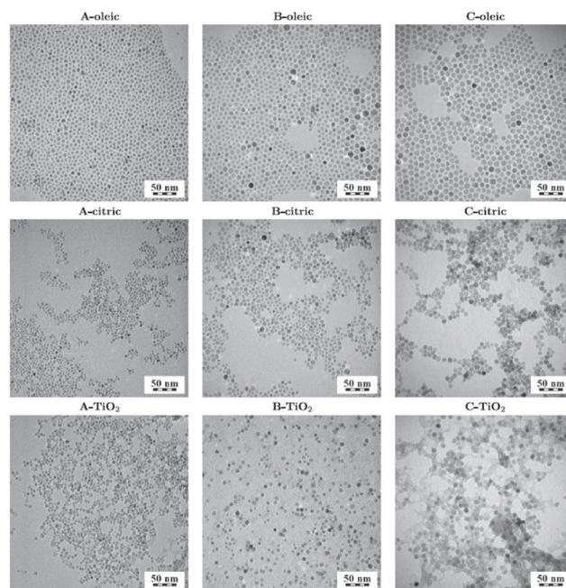
Fig. 9  $CoFe_2O_4$  crystallites of three different sizes (A, B and C) coated with oleic acid, citric acid and  $TiO_2$ . Reproduced with permission from Repko *et al.*<sup>220</sup>
