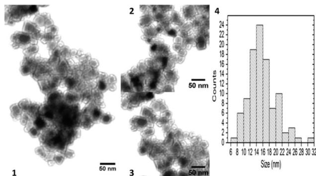
Fig. 14 TEM micrographs and size histogram of Ni<sub>0.4</sub>Cu<sub>0.2</sub>Zn<sub>0.4</sub>Fe<sub>2</sub>O<sub>4</sub> synthesised at  $T = 90$  °C,  $t = 2$  h and for  $P_{\text{diss}} = 46.27$  W (1, 2, and 3 represent different areas of the sample; 4 the size histogram). Reproduced with permission from Harzali *et al.*<sup>266</sup>
