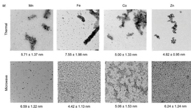
**Fig. 18** TEM images of MFe<sub>2</sub>O<sub>4</sub> nanoparticles synthesized by the thermal and microwave synthetic routes. For all the investigated cases, the microwave synthesis produces highly homogeneously dispersed nanoparticles. The numbers below each image display the average nanoparticle size with its deviation. Reproduced with permission from Solano *et al.*<sup>331</sup>
