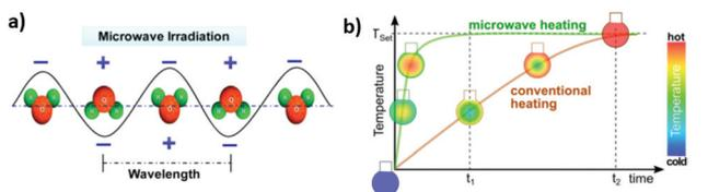
**Fig. 16** (a) Water molecules in an alternating electrical field under microwave irradiation (from ref. 323) (b) Time–temperature correlation of conventional and MW-heated reaction vessels as well as the temperature distribution inside the reaction mixture. Reproduced with permission from Schütz *et al.*<sup>324</sup>
