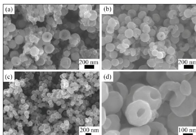
**Fig. 11** Scanning electron microscopy images of CoFe<sub>2</sub>O<sub>4</sub> nanospheres prepared *via* hydrothermal synthesis in the presence of ethylene glycol at reaction times of (a) 6 hours, (b) and (d) 12 hours and (c) 24 hours. Reproduced with permission from Wang *et al.*<sup>232</sup>
