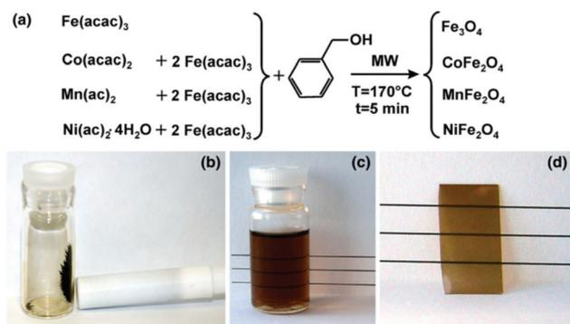
**Fig. 19** (a) General reaction scheme displaying the metal oxide precursors employed in the sol-gel synthesis, the solvent, the experimental conditions, and the final composition of the nanoparticles. Photographs of (b) magnetite nanopowder under the influence of a permanent magnet, (c)  $\text{CoFe}_2\text{O}_4$  dispersion in ethanol, and (d)  $\text{CoFe}_2\text{O}_4$  film on a glass substrate. Reproduced with permission from Bilecka *et al.*<sup>342</sup>
