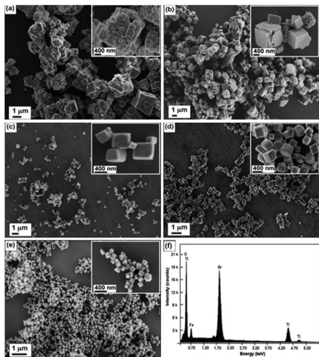
**Fig. 20** SEM images of  $\text{SrTi}_{1-x}\text{Fe}_x\text{O}_3$  samples prepared *via* microwave-assisted hydrothermal method:  $x = 0.0$  (a),  $0.05$  (b),  $0.1$  (c),  $0.25$  (d),  $0.4$  (e); (f) EDX spectrum of the  $x = 0.25$  sample. Reproduced with permission from da Silva *et al.*<sup>345</sup>
