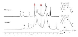
Fig. 2 <sup>1</sup>H NMR spectra of PFP-polymer (top) and PFP-SCNP (below) in acetone-d<sub>6</sub>, indicating the appearance of crosslinker and endcap signals.
