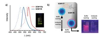
Fig. 4 (a) Emission (solid line) and excitation spectra (dotted line) of SCNP-F3a (blue, with inset) and SCNP-F8 (red); (b) schematic representation of the elution of SCNP-F7 and SCNP-F8 from a Ni<sup>2+</sup>-NTA column and image of the two elution fractions of SCNP-F8 under UV irradiation  $(\lambda = 365 \text{ nm}).$
