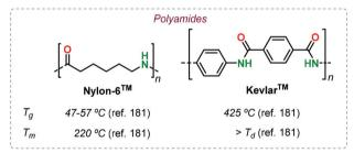
Fig. 30 Thermal properties of representative petroleum-based commercial polymers.
