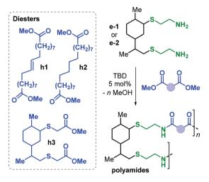
Fig. 26 Synthesis of limonene-based polyamides poly(e-alt-h).
