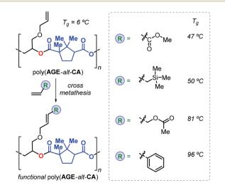
Fig. 19 Functional polymers derived from poly(AGE-alt-CA) after postmodification using cross-metathesis reactions.
