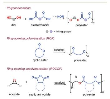
**Fig. 9** Aliphatic polyester synthesis by polycondensation and ring-opening (co)polymerisation.
