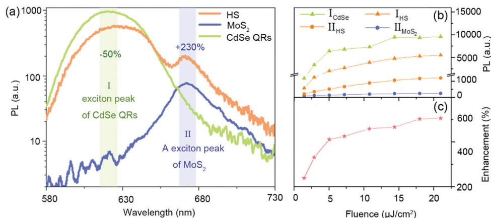
Fig. 2 (a) PL spectra of heterostructure (orange), pristine MoS<sub>2</sub> monolayer (blue), and CdSe QRs (green). (b) PL intensity of all of the heterostructure, MoS<sub>2</sub>, and CdSe QRs. (c) PL enhancement of MoS<sub>2</sub> as a function of incident fluence. Defining  $I_{\text{HS}}/I_{\text{MoS}_2}$  as PL enhancement.
