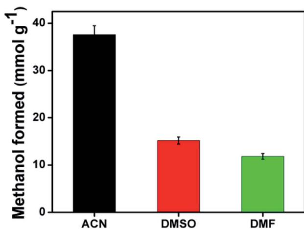
Fig. 10 Influence of the reaction medium for the production of methanol from CO<sub>2</sub> reduction under visible light by 5.0rGO-TiO<sub>2</sub> for a period of 16 h. Reproduced with permission from Mungse *et al.*, 2015. Copyright 2015, Royal Society of Chemistry.
