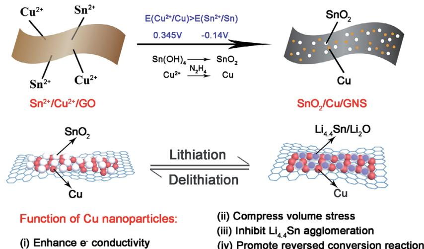
Fig. 2 Schematic illustration of the selective reduction fabrication of  $\text{SnO}_2/\text{Cu}/\text{GNS}$  composite; structure evolution and functions of Cu nanoparticles during lithiation and delithiation processes. Reproduced with permission from Jiang *et al.*, 2019. Copyright 2019, Elsevier.
