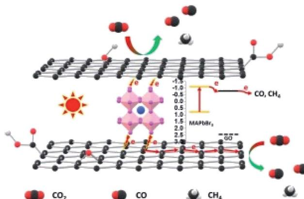
Fig. 12 Possible mechanistic pathway of photoelectrochemical CO<sub>2</sub> reduction. Reproduced with permission from Wang *et al.*, 2018. Copyright 2018, Elsevier.
