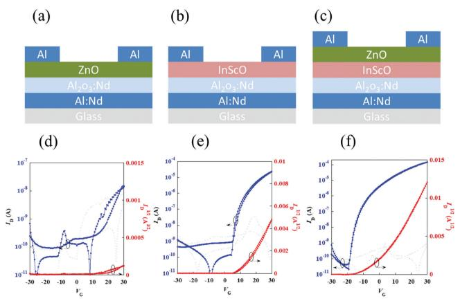
Fig. 1 (a-c) The device structure of the TFTs with solution-processed ZnO-nanoparticle, InScO and InScO/ZnO-nanoparticle heterojunction (with optimized thicknesses of 3.4 nm/50 nm) channels by spin-coating, respectively. (d-f) The transfer characteristics of TFTs with different channels measured at  $V_{DS} = 30$  V and  $V_{GS} = -30$  to 30 V.
