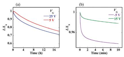
Fig. 5 (a) The operational lifetime of the red QD-HLET tested at different  $V_{GS}$  and a constant current density of 71 mA cm<sup>-2</sup>. (b) The luminance as a function of time for the red QD-HLET with a loop test between -5 V and 15 V of  $V_{GS}$  at a constant current density of 71 mA cm<sup>-2</sup>.
