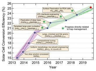
Fig. 5 Overview of recent progress in single junction perovskite solar cell efficiency, identifying the key technological advances.<sup>59–61,75,80,120,134,137,138</sup> The red circle indicates the current record (25.2%) confirmed by National Renewable Energy Laboratory (NREL). 139
