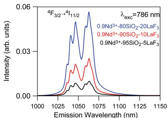
Fig. 10 Emission spectrum of 450 °C–6 h 0.9Nd<sup>3+</sup>–SiO<sub>2</sub>:LaF<sub>3</sub> GCs with three different crystalline fractions 5% (black), 10% (red) and 20% (blue) obtained under 786 nm excitation.
