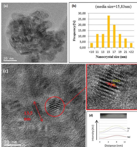
Fig. 6 (a) HRTEM image of  $0.9\text{Nd}^{3+}\text{-LaF}_3$  nanoparticles in the  $0.9\text{Nd}^{3+}\text{-80SiO}_2\text{:}20\text{LaF}_3$  sol. (b) Distribution of nanocrystal size of the nanoparticles in the sol. (c) EDX of the corresponding  $0.9\text{Nd}^{3+}\text{-LaF}_3$  nanoparticle and its scanning lines. (d) STEM analysis of the corresponding  $0.9\text{Nd}^{3+}\text{-LaF}_3$  nanoparticle and its scanning lines.
