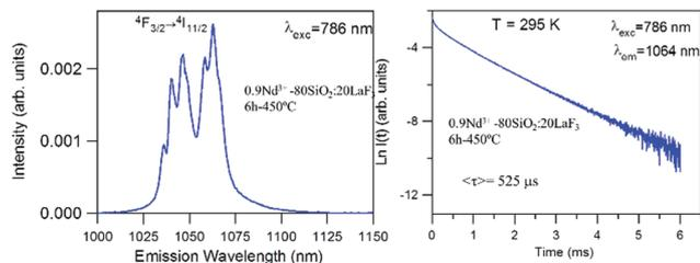
Fig. 9 Emission spectrum of 450 °C–6 h 0.9Nd<sup>3+</sup>–80SiO<sub>2</sub>:20LaF<sub>3</sub> sol and its corresponding semi-logarithmic plot of the experimental decay under excitation at 786 nm collecting the luminescence at 1064 nm.
