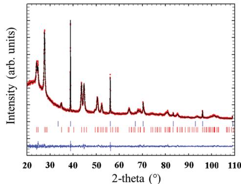
Fig. 7 Observed (red circles), calculated (continuous black line) and difference (continuous blue line) X-ray diffraction profiles of  $0.9\text{Nd}^{3+}\text{-80SiO}_2\text{:}20\text{LaF}_3$  particulate sol powders treated at  $450\text{ }^\circ\text{C}$  for 6 h with 5% NaF as internal standard. The Bragg peaks of NaF and  $\text{LaF}_3$  are indicated by top and bottom vertical bars, respectively.
