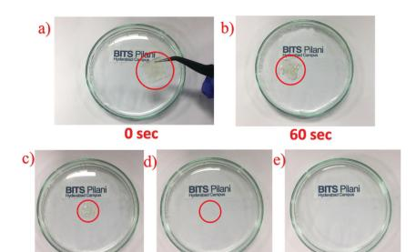
Fig. 8 Images of different stages of dissolution of SnS<sub>2</sub> QDs with the PVA substrate in DI water: (a) 0 s, (b) 60 s, (c) 180 s, (d) 300 s and (e) 360 s.
