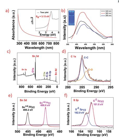
Fig. 3 (a) UV-Visible absorption spectra of SnS<sub>2</sub> QDs; the inset is the Tauc plot showing a bandgap of  $\sim 3.13$  eV. (b) Photoluminescence spectra of SnS<sub>2</sub> QDs at different excitation from 345 nm to 390 nm. (c) XPS survey spectra of SnS<sub>2</sub> QDs. (d) High resolution spectra of C 1s. (e) High resolution spectra of Sn 3d. (f) High resolution spectra of S 2p.
