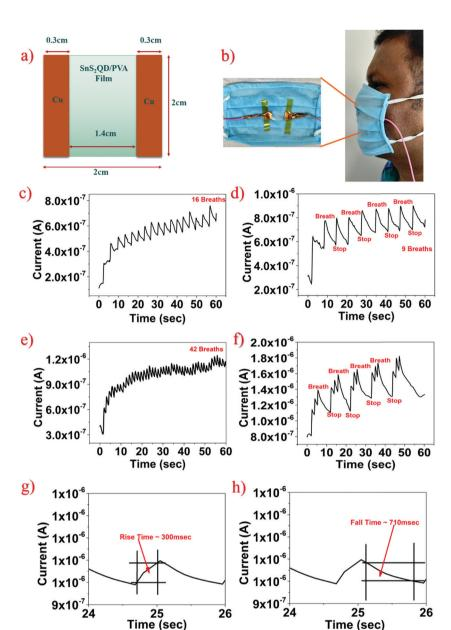
Fig. 6 (a) Schematic of a breath sensor. (b) Integration of the sensor in the breath mask. (c) Continuous-time response of  $SnS_2$  QD/PVA under normal breath. (d and e) Slow and fast breath patterns over a period of 60 seconds. (f) Three breath iterative breathing patterns for five cycles. (g and h) The rise time and fall time of the fabricated sensor were  $\sim 300$  ms and  $\sim 710$  ms.
