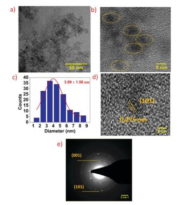
Fig. 2 (a and b) TEM image of the synthesized SnS<sub>2</sub> QDs, (c) size distribution of SnS2 QDs, calculated average diameter of SnS2 QDs is  $3.99 \pm 1.58$  nm, (d) HRTEM lattice fringes of SnS $_2$  QDs, and (e) SAED pattern of SnS2 QDs.
