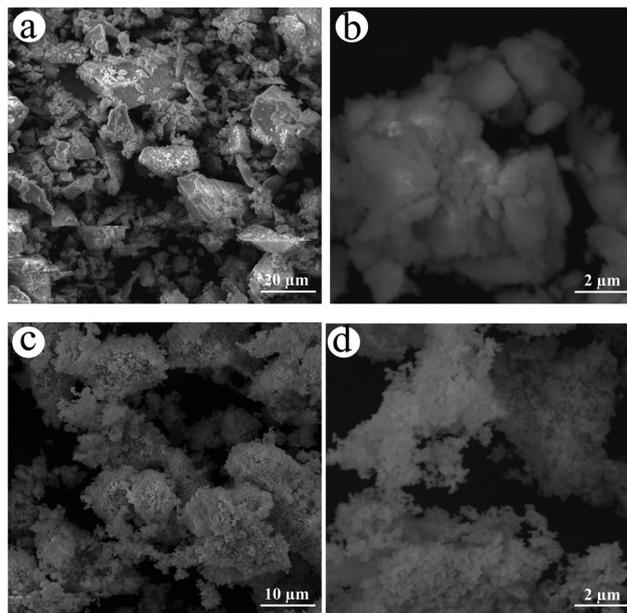
Fig. 3 SEM images for (a)  $\text{CoWO}_4$  (low magnification), (b)  $\text{CoWO}_4$  (high magnification), (c)  $\text{Ni-CoWO}_4$  (low magnification), and (d)  $\text{Ni-CoWO}_4$  (high magnification).
