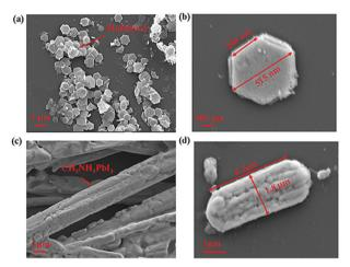
Fig. 2 (a and b) SEM image of the CH<sub>3</sub>NH<sub>3</sub>Pbl<sub>3</sub> perovskite prepared at room temperature; (c and d) SEM image of the CH3NH3PbI3 perovskite prepared at 80 °C
