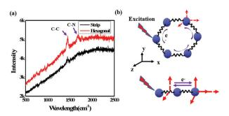
Fig. 8 (a) Raman spectra of different shaped CH<sub>3</sub>NH<sub>3</sub>Pbl<sub>3</sub> perovskites and (b) schematic illustration of the Raman scattering for different shaped CH<sub>3</sub>NH<sub>3</sub>Pbl<sub>3</sub> perovskites.
