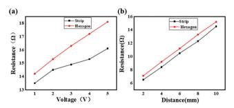
Fig. 11 (a) Resistance-voltage curves of the two different shaped CH<sub>3</sub>NH<sub>3</sub>Pbl<sub>3</sub> perovskites on ITO glass substrates and (b) resistances of the two different shaped CH3NH3Pbl3 perovskites on ITO glass, with the length of the ITO glass ranging from 2 mm to 10 mm
