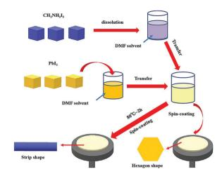
Fig. 1 Schematic illustration of the fabrication of the CH<sub>3</sub>NH<sub>3</sub>Pbl<sub>3</sub>
