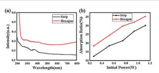
Fig. 9 (a) UV-vis spectra of two different shaped CH<sub>3</sub>NH<sub>3</sub>Pbl<sub>3</sub> perovskites and (b) absorption measurement of two different shaped CH3NH3Pbl3 perovskites, subjected to an incident laser with a wavelength of 468 nm.
