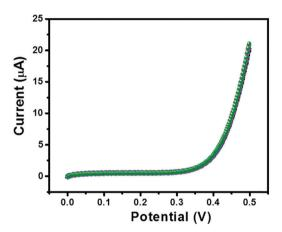
Fig. 12 Five consecutive I-V curves of GC-2 in the presence of urea  $(250 \mu M)$  in 0.1 M PBS (pH = 7.0).
