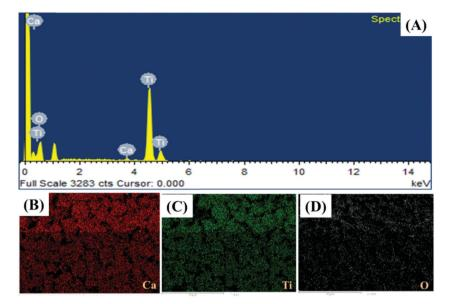
Fig. 4 EDX analysis of CaTiO<sub>3</sub> pyramids.
