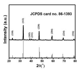
Fig. 1 PXRD pattern of CaTiO<sub>3</sub> pyramids
