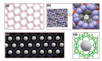
Fig. 7 (a) Expanded 3D model of MOF-1. (b) Space filled model of MOF-1 showing a single unit of the expanded MOF-1. (c) and (d) Space occupied by the MB structure in the 3D MOF-1. (25 Reproduced from ref. 125 with permission from Springer.
