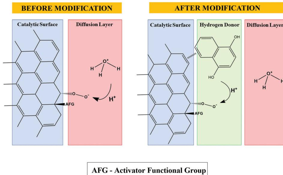
Fig. 2 Proposed scheme for the unmodified carbon surface and incorporation of the organic compound 1,4-naphthoquinone, which acts as an H<sup>+</sup> donor for the ORR.
