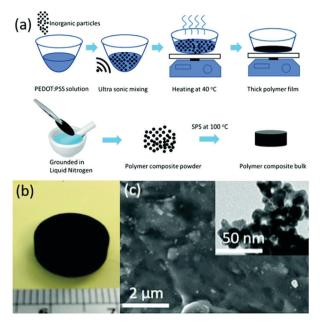
Fig. 5 (a) Process used to synthesize bulk polymers. (b) Photograph of a polymer bulk sample after applying SPS. (c) CSS polymer bulk with an inset showing a TEM image of Cu<sub>2</sub>SnSe<sub>3</sub> nanoparticles. (Reproduced from ref. 56 with permission from The Royal Society of Chemistry.).
