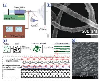
Fig. 4 (a) Scheme of a conventional electrospinning setup, <sup>39</sup> (b) electrospun hollow PbTe nanofibers, 44 (c) schematic of the formation mechanism and (d) SEM image of CNT/PANI nanofibers.<sup>45</sup>
