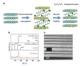
Fig. 2 (a) Schematic of the electrochemical intercalation process. (b) XRD patterns of  $TiS_2$  single crystal and its related superlattice structures. (c) Magnified STEM image of  $TiS_2$ (HA)<sub>0.025</sub>. (Reproduced from ref. 33 with permission from Nature Communication.).
