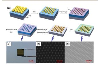
Fig. 9 (a) Scheme of the fabrication of the organic/inorganic hybrid film via by nanosphere lithography, (b) digital photograph of closely packed monolayer PS nanospheres on a SiO<sub>2</sub>/Si substrate after etching, SEM image of (c) Bi<sub>2</sub>Te<sub>3</sub> nanoparticle arrays prepared by using 100 nm PS nanospheres as patterns and (d) PEDOT/Bi<sub>2</sub>Te<sub>3</sub>(100) hybrid films. 109
