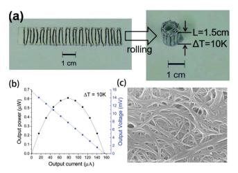
Fig. 10 (a) Photograph and (b) output power-current and output voltagecurrent curves of the TEG with SWCNT/PVDF composite fibers. (c) SEM image of PEI(2wt%)-treated SWCNT/PVDF fibers (50wt%). (Reproduced from ref. 135 with permission from The Royal Society of Chemistry.).
