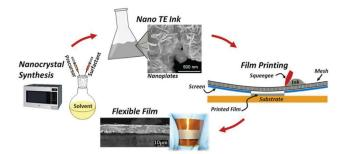
Fig. 6 Schematic of the overall fabrication process of flexible thermoelectric films, including nanocrystal synthesis, nano-ink processing, screen printing of thermoelectric films on a flexible substrate, and sintered flexible films. (Reproduced from ref. 63 with permission from Scientific Reports.).
