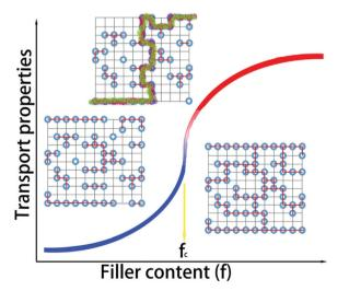
Fig. 1 Percolation theory and nonlinear changes in the transport properties of composites near the percolation threshold  $f_c$  (dashed blue line). The insets show the geometric phase transition of fillers (denoted by dark spots) in the microstructures of the composites near percolation.
