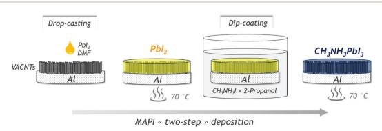
Fig. 1 Scheme of the two-step process used for MAPI deposition
