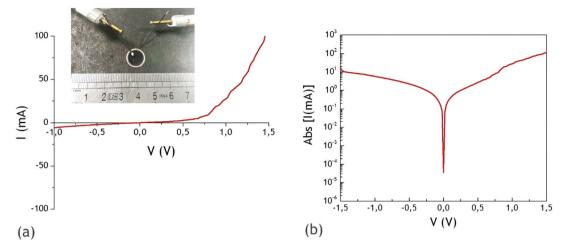
Fig. 6 (a) I–V dark measurment of Al/VACNTs/ZnO/perovskite/spiro-OMeTAD/EGa:In device – 0.0079 cm<sup>2</sup> active area and (b) semi-logarithmic representation.
