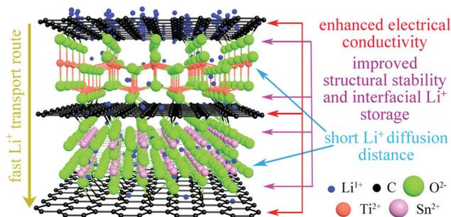
Fig. 8 A schematic illustration of the lithium ion storage mechanism in the  $\text{SnO}_2@\text{TiO}_2/\text{C}$  nanoarchitecture.
