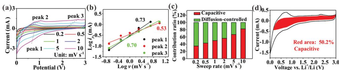
Fig. 6 (a) CV curves at different scanning rates; (b) the line relationship of  $\log(i)$  vs.  $\log(\nu)$  at peaks 1–3 marked in (a); (c) the percentages of the pseudocapacitive contribution at different scanning rates; and (d) the detailed pseudocapacitive contribution at a scanning rate of 1 mV s<sup>-1</sup> of SnO<sub>2</sub>@TiO<sub>2</sub>/C.
