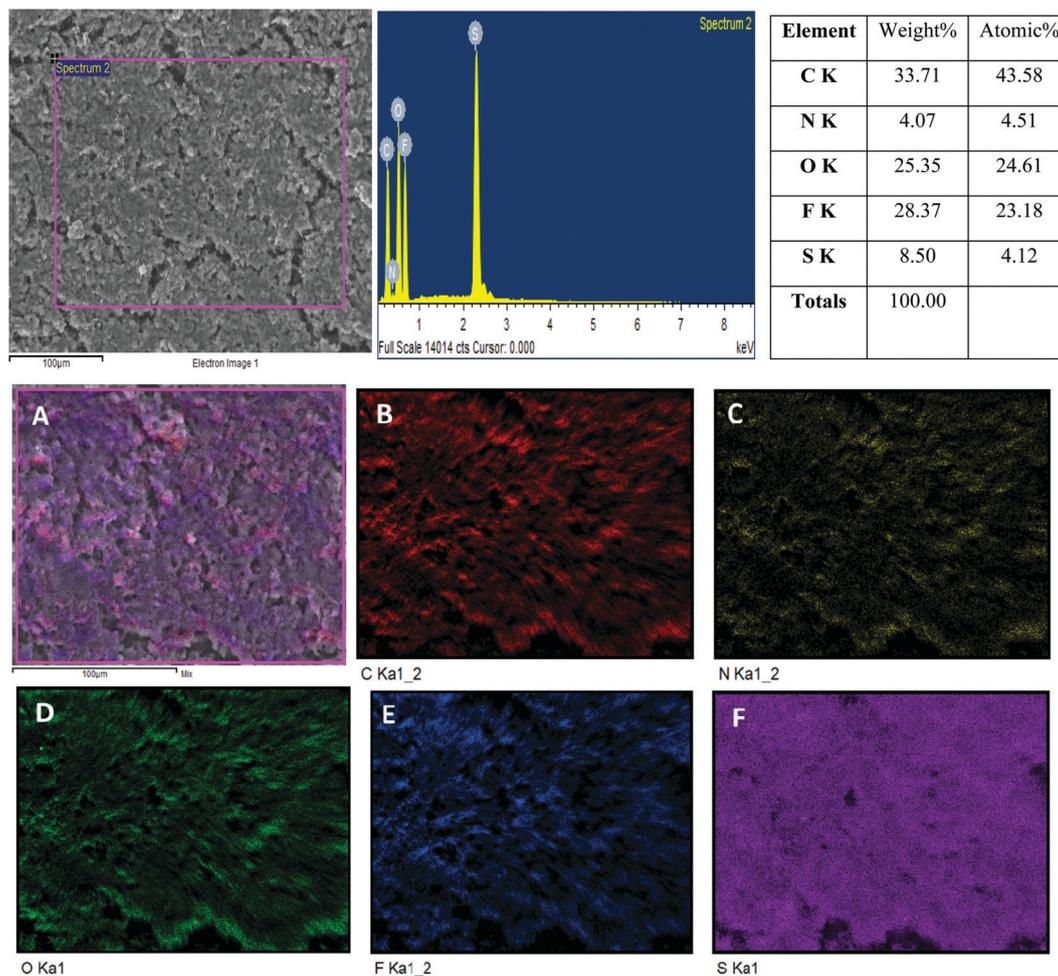
Fig. 8 Panel (1): the EDS spectrum of the POP coated membrane after cycling; panel 2 and 3: (A) the FE-SEM image of the POP coated membrane and elemental mapping of (B) carbon, (C) nitrogen, (D) oxygen, (E) fluorine and (F) sulfur after cycling.
