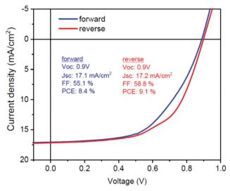
Fig. 4 J-V characteristics of a photovoltaic cell with an area of 1.5 cm<sup>2</sup> with four layers of the stack deposited by inkjet printing. The device shows little hysteresis from reverse to forward scan.
