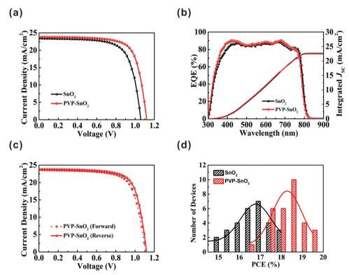
Fig. 5 (a) J-V curves of the best-performing perovskite solar cells using the SnO<sub>2</sub> and PVP-SnO<sub>2</sub> ETLs measured under reverse scans. (b) The external quantum efficiency (EQE) spectra and the corresponding integrated  $J_{SC}$  curves for the best-performance PSCs with different ETLs. (c) J-V curves of devices using the PVP-SnO<sub>2</sub> ETL under reverse and forward scans. (d) The PCE distribution histogram of the planar type PSCs with different ETLs.
