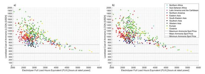
Fig. 2 2019 Scenario – Range of the optimal achievable LCOA and the respective electrolyser full load hours equivalent (FLH) grouped by geographic region for a (a) multi-national and (b) domestic corporation. Benchmarked against the maximum, mean and minimum of 2000–2019 NOLA, Black Sea, Middle East, Western Europe and US Tampa ammonia spot prices (720, 426 and \$165  $t^{-1}$  respectively). Estimates above \$2000  $t^{-1}$  are not presented due to prioritisation of lower estimates.
