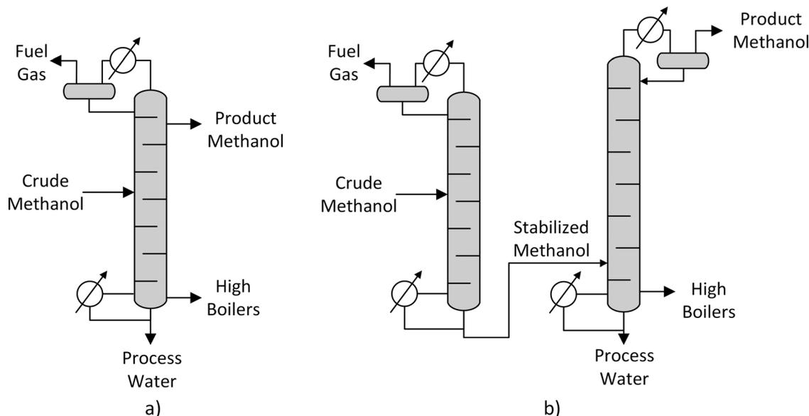
Fig. 8 Single column (a) and two-column (b) methanol distillation, own illustration based on Supp.<sup>55</sup>
