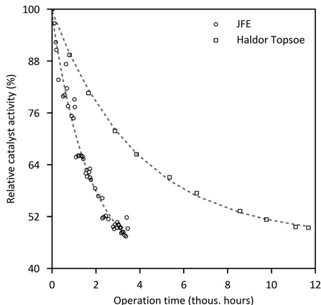
Fig. 14 Deactivation of direct DME synthesis catalysts of Haldor Topsøe<sup>130</sup> and JFE (260 °C, 50 bar).<sup>258</sup>
