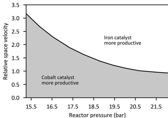
Fig. 22 Productivity comparison between iron (240 °C) and cobalt (220 °C) based catalysts. Adapted from Steynberg and Dry.<sup>35</sup>
