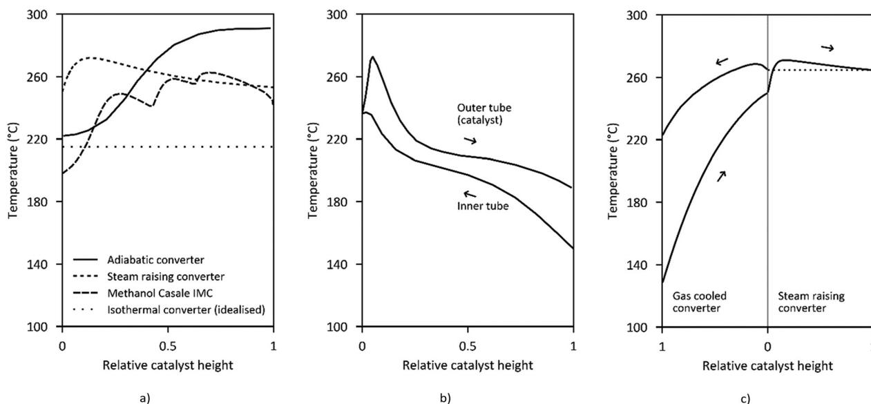
Fig. 7 Temperature profiles along the reactor length of (a) adiabatic converter,<sup>105</sup> steam raising converter,<sup>126</sup> Methanol Casale IMC,<sup>142</sup> and isothermal converter (idealized), (b) Mitsubishi Superconverter,<sup>143</sup> (c) Lurgi MegaMethanol.<sup>99</sup>
