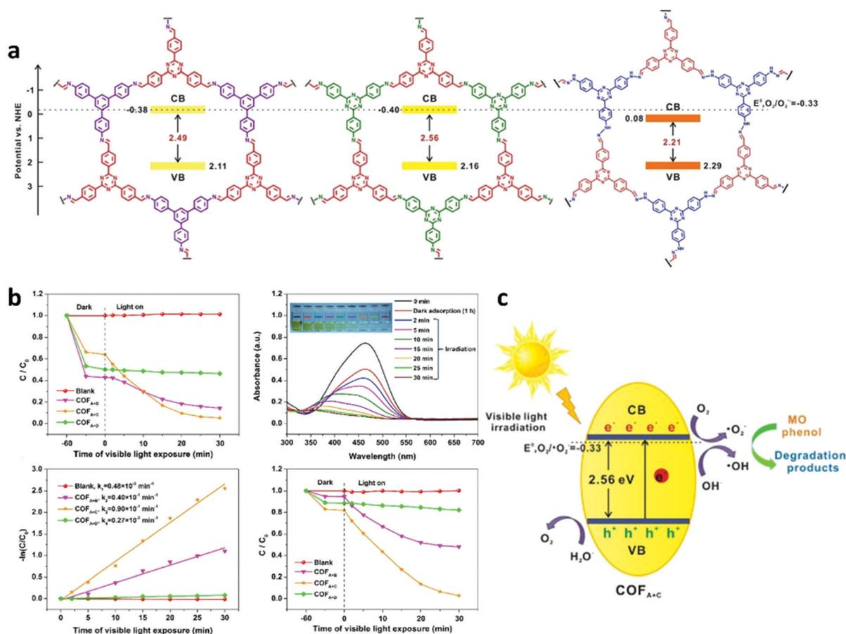
Fig. 15 (a) Structure and band alignment of  $\text{COF}_{\text{A+B}}$ ,  $\text{COF}_{\text{A+C}}$  and  $\text{COF}_{\text{A+D}}$ . (b) Photocatalytic performance of  $\text{COF}_{\text{A+B}}$ ,  $\text{COF}_{\text{A+C}}$  and  $\text{COF}_{\text{A+D}}$  under visible light irradiation. (c) Schematic illustration of pollutant photodegradation over  $\text{COF}_{\text{A+C}}$  under visible light irradiation. Reproduced with permission from ref. 253. Copyright 2017, Elsevier B. V.
