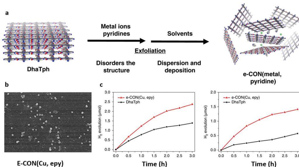
Fig. 7 (a) Scheme for the preparation of e-CON. (b) SEM image of e-CON (Cu, epy) deposited on the silicon wafer. (c) H<sub>2</sub> evolution upon irradiation with visible (>420 nm) and NIR (>780 nm) light using e-CON(Cu, epy)/Pt/RGO and DhaTph/Pt/RGO. Reproduced with permission from ref. 163. Copyright 2019 Springer Nature Limited.
