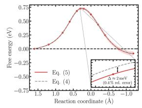
Fig. 6 Comparison of free energy profiles of the Volmer reaction determined from the bare force of constraint, egn (5), and the unbiased solvent averaged force, egn (4). The results correspond to simulations performed within the unrestrained ensemble
