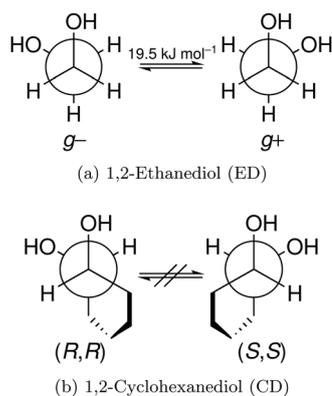
**Fig. 1** Newman projections of ED (a) and CD (b). The projections illustrate how interconversion of the ED enantiomers is possible whereas the cyclohexyl backbone demands a tetrahedral carbon inversion or similarly thermally demanding processes. The barrier was calculated at the B3LYP-D3/def2-QZVP level including zero point energy.
