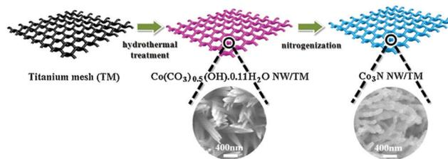
Fig. 14 Schematic diagram of  $\text{Co}_3\text{N}$  NW/TM synthesis. Reproduced ref. 180 with permission from Elsevier B.V., copyright 2017.
