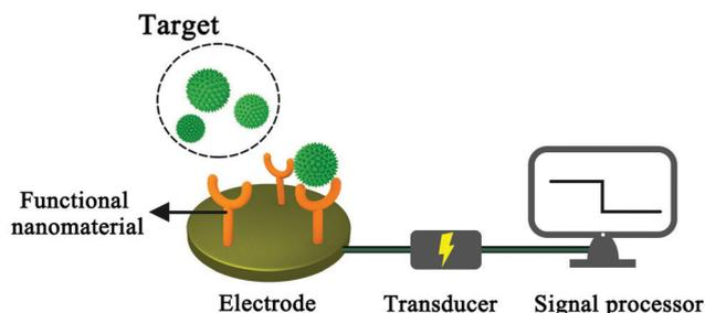
Fig. 1 Schematic diagram of an electrochemical sensor.
