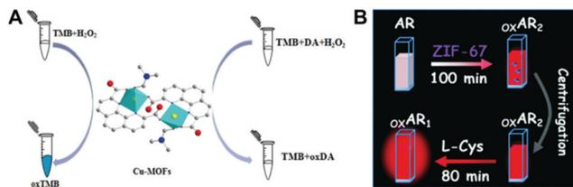
**Fig. 13** (A) Presents the strategy for DA detection based on the target impacting the peroxidase-like Cu-MOF catalyzed TMB color reaction (reused with permission from ref. 34). (B) shows the sensing principle for L-Cys based on oxidase-mimicking ZIF-67 catalyzed AR oxidation (reused with permission from ref. 47).
