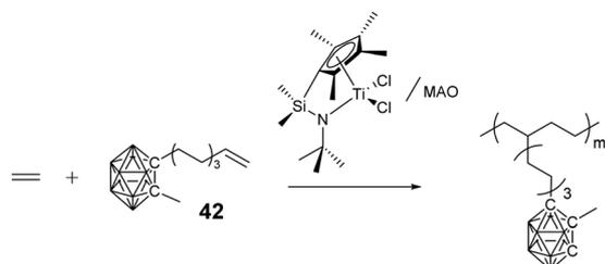
Fig. 11 Linear BCCPs prepared through coordination polymerization.
